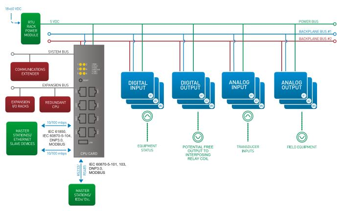
The RTU System Bus allows expansion of the RTU communication capabilities. The system bus consists of a 16bit high speed parallel bus and high speed serial bus. These busses allows installation of communication extender modules or specialty modules, which provide additional serial/Ethernet interfaces and/or specific function like LON interfaces.
