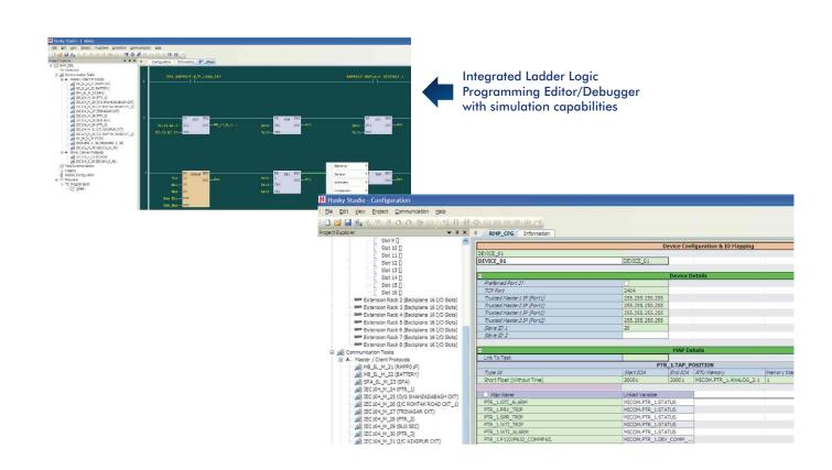
HUSKY Studio is a powerful configuration editor designed for Data Concentrators where large amount of data is transferred across protocols using IO maps. Features like variable naming, filtering allow configuration engineer to map the data across protocols by referring to user friendly names. Built in Event Viewer allows you to view different events, with millisecond timestamp, in the RTU itself.
