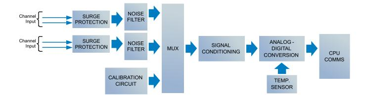
Analog Input module provides different input ranges to suit most types of applications. Each channel is individually configurable for voltage and current (via hardware jumpers) and each channel can be further configured for different input ranges to suit the application requirement. Input ranges are configurable from Husky Studio.
